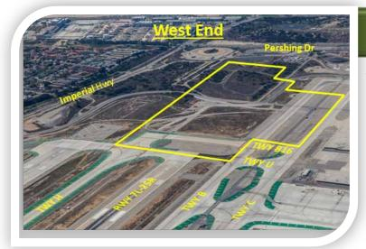
This project will provide safety improvements to the Runway Safety Area (RSA) at the west end of Runway 25R/7L to meet the latest FAA standards. The west end of the runway will provide the full 1,000 feet clearance for the RSA. The project will also replace deteriorated concrete pavement at the east end of Runway 25R/7L.
