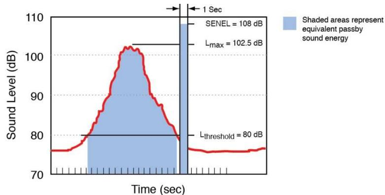
Because SENEL is a cumulative measure, a higher SENEL can result from either a louder or longer event, or some combination. Figure G-6 provides a representative example: The longer duration noise event on the right results in a higher SENEL than the event on the left, even though it has a lower Lmax.
