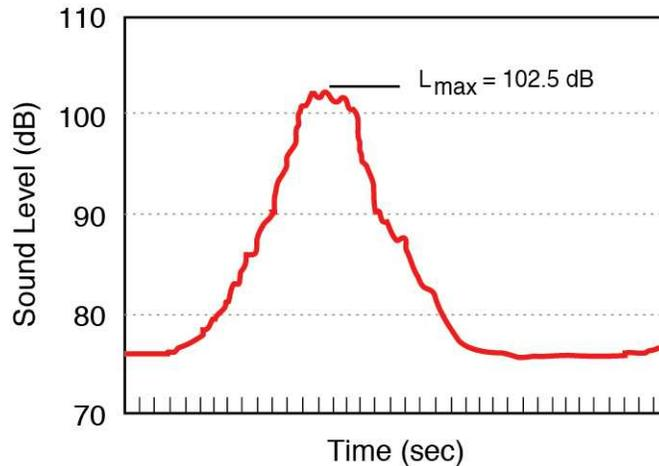
Because of this variation, it is often convenient to describe a particular noise "event" by its maximum sound level, abbreviated as  $L_{max}$ . In Figure G-3 the  $L_{max}$  is approximately 102.5 dB.
