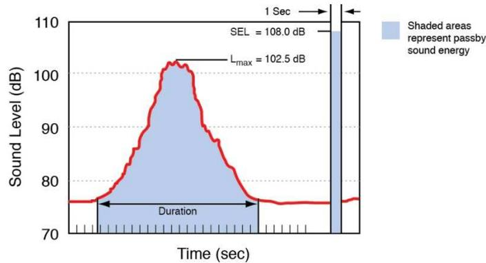
Note that because SEL is normalized to one second, it almost always will be a higher value than the event's  $L_{max}$ . In fact, for most aircraft flyovers, SEL is on the order of five to 12 dB higher than  $L_{max}$ .
