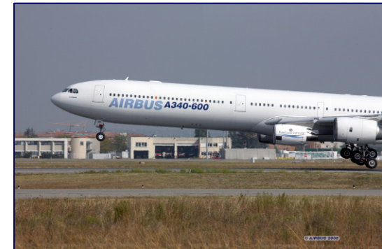
A340-600 Flying Test Bed 27 Flights 76 Hours
