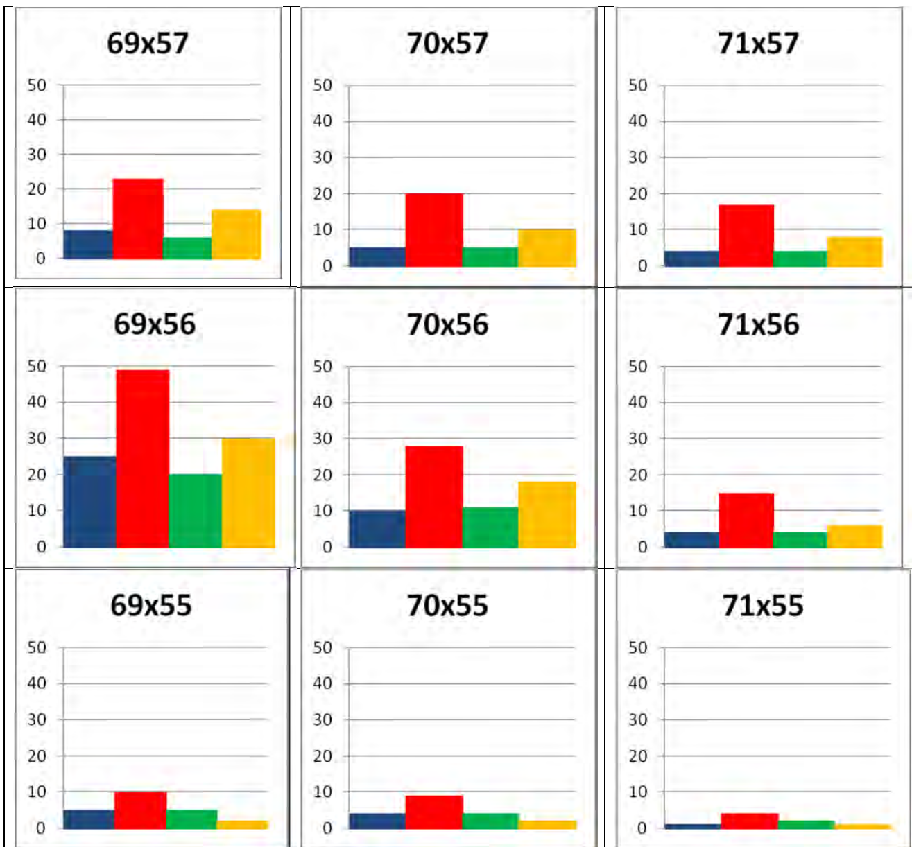
Figure 10-8. Incremental airport-related contribution above background modeled by CMAQ during the Summer Season (as percentage increase over background). The numbers at the top of each graph represent the corresponding grid cell as seen in Figure 10-6.
