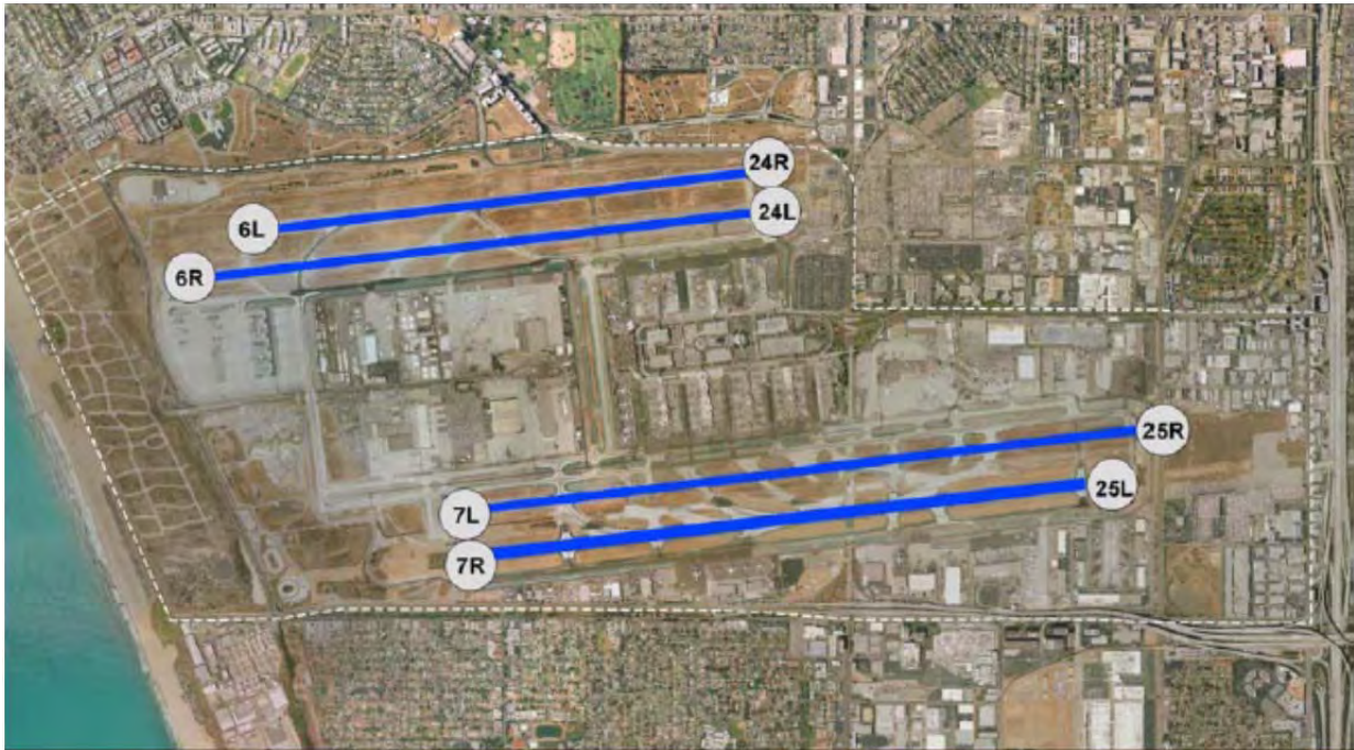
Figure 8-2. The North and South Airfields for LAX. The North Airfield consists of Runways 6R/6L and 24R/24L. The South Airfield consists of Runways 7R/7L and 25R/L.
