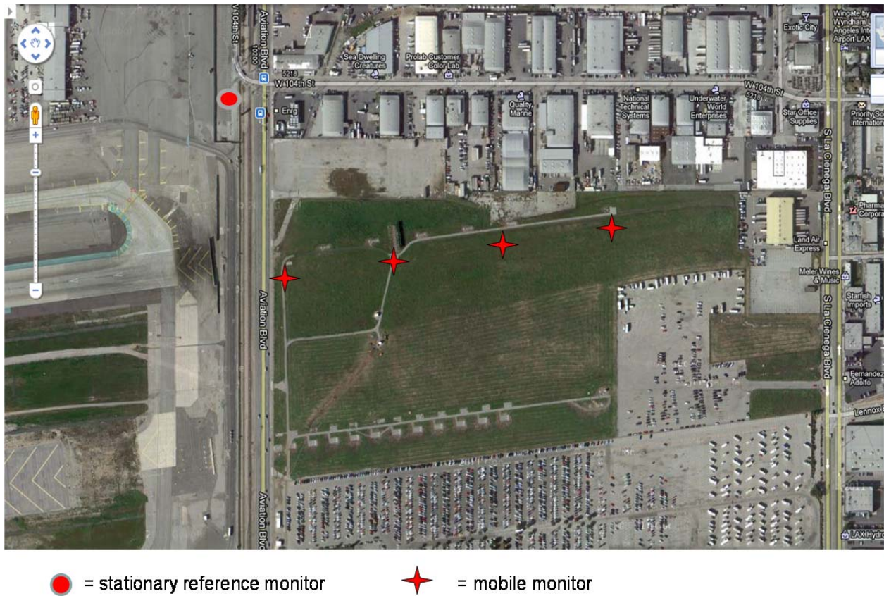
Figure 5. Survey #2 - South Runway/Aviation Boulevard West-East Gradient. Field between Aviation and La Cienega is 160 to 800 meters east of the east end of Runway 25R.
