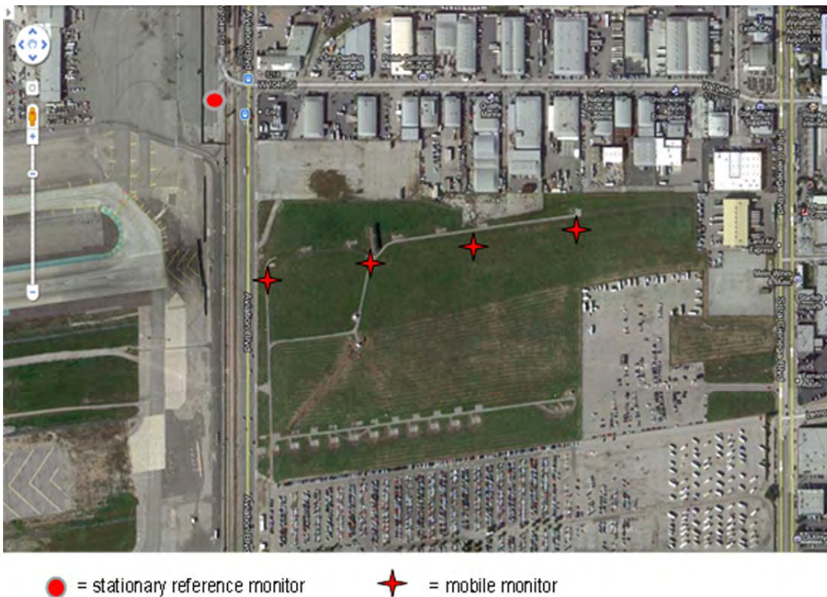
Figure 5-9. South Runway/Aviation Boulevard. West-East Gradient. Field between Aviation Boulevard and La Cienega Boulevard is 160 to 800 meters east of the east-end of South Airfield Runway 25R.
